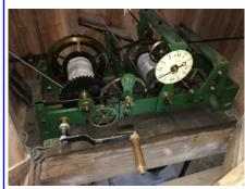
physical connection between the hour hand and the number of chimes, which is why sometimes it may strike the wrong number of chimes! When the clock reaches the hour, a lever is activated which pulls on a series
