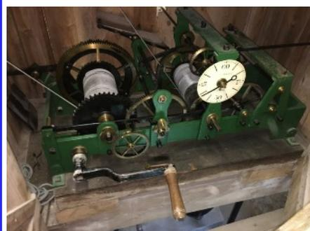
physical connection between the hour hand and the number of chimes, which is why sometimes it may strike the wrong number of chimes! When the clock reaches the hour, a lever is activated which pulls on a series
